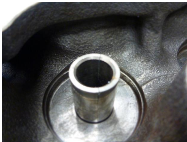
Figure 6. Cracks in valve guides
