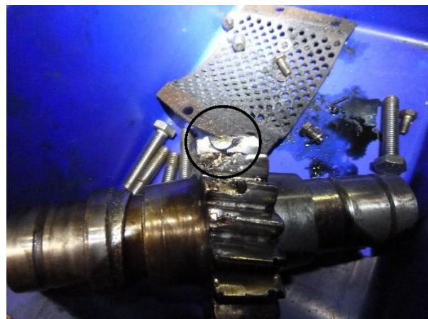
Figure 2 Ball bearing shaped hole in gear tooth
