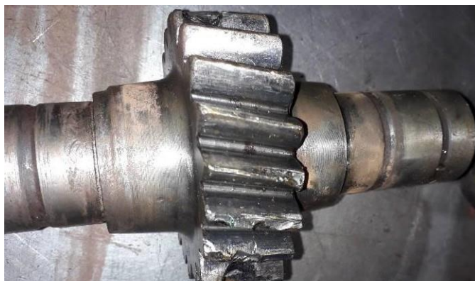
Figure 9: Driveshaft for hydraulic pump showing damage to the teeth
