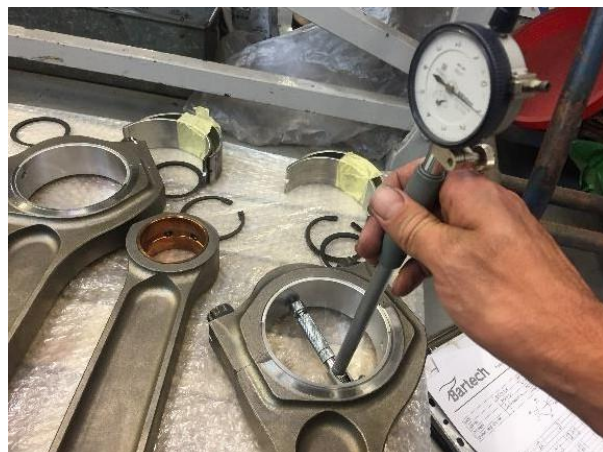
Figure 6. Inspection of large end with shells fitted
