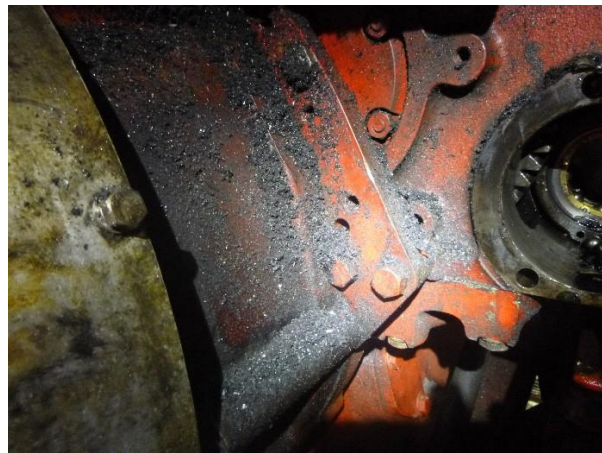
Figure 4 Swarf around hole in crankcase
