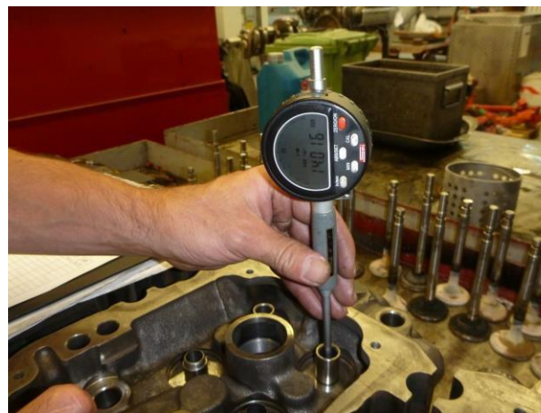
Figure 8. Valve guide bore measured
