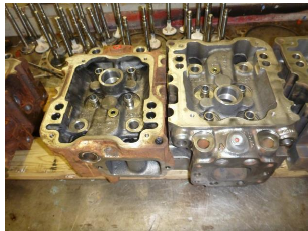
Figure 4. MPI crack testing of all heads
