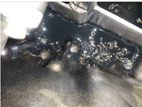
Figure 10. Broken gears in sump
