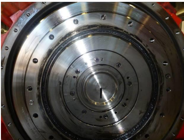
Figure 8. Flywheel marked and removed
