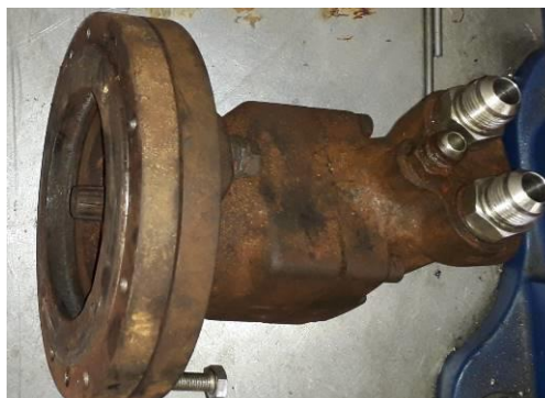
Figure 12: Hydraulic pump, the spline shaft has been bent in the failure.
