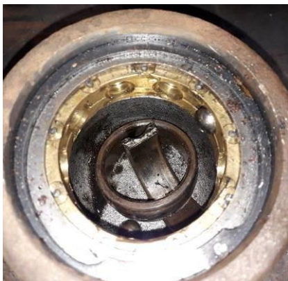
Figure 8: Damaged rear bearing
