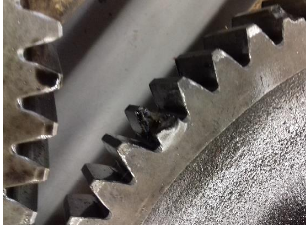
Figure 4. Ball bearing shape hole in teeth
