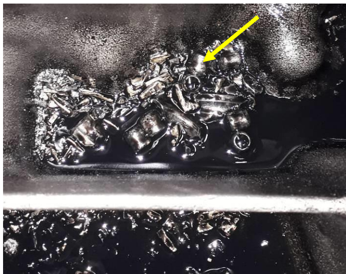
Figure 6. Showing debris in sump
