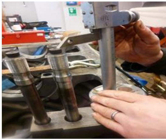
Figure 2. Studs reset to specified length
