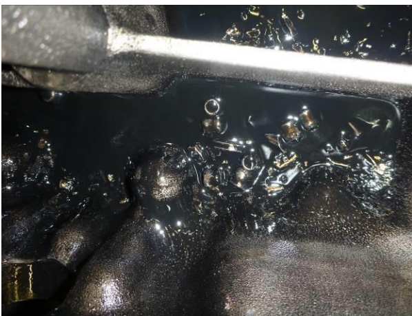
Figure 8. Broken gears & swarf in sump
