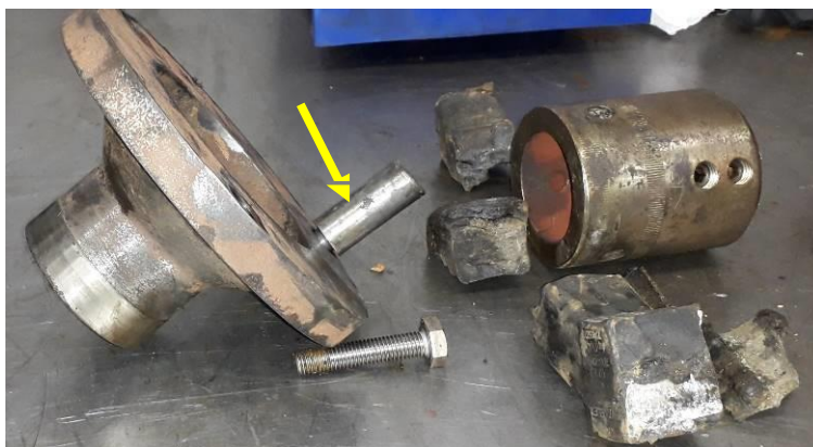
Figure 11: Damaged rubber coupling, drive coupling (Left) shows a broken bolt still in situ
