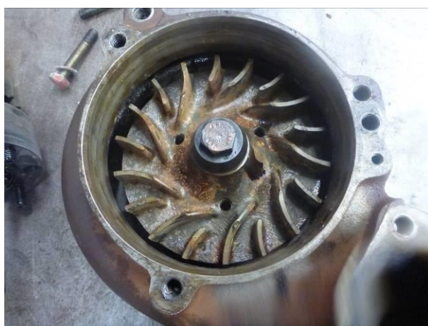
Figure 3. No damage to impeller
