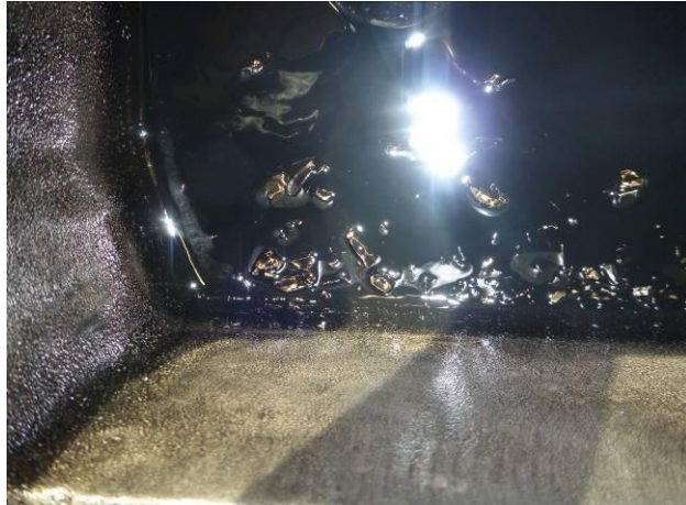
Figure 9. Broken gears in sump
