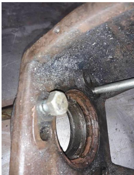
Figure 10: Damaged front bearing housing
