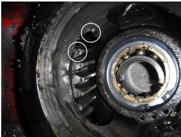
Figure 3 Damage to idler teeth and crankcase
