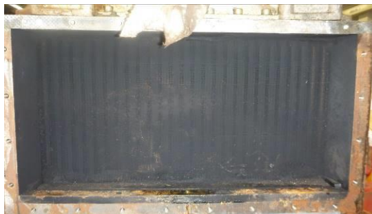
Figure 2: Showing excessing carbon build up on Intercooler
