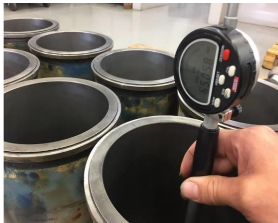
Figure 6. Measuring of the ovality
