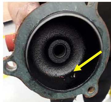
Figure 3: Small sections of bearing were found on fuel lift pump adaptor
