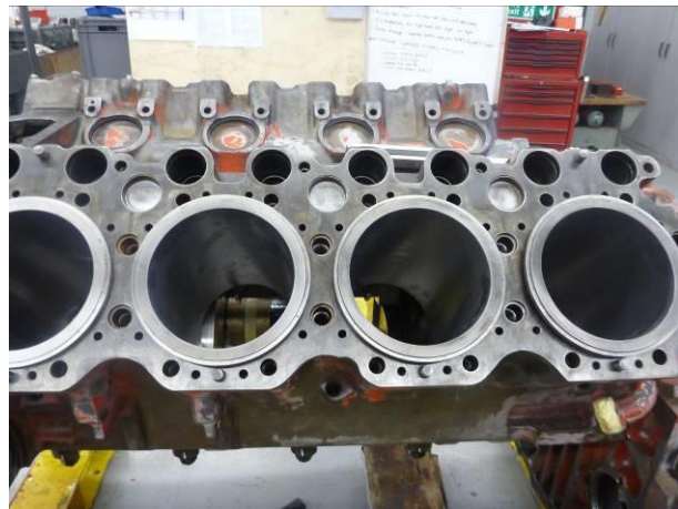
Figure 11. Crankcase chemically cleaned
