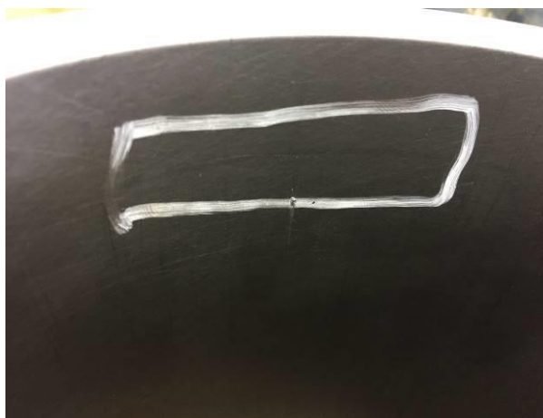
Figure 2. Ridge at top of ring travel
