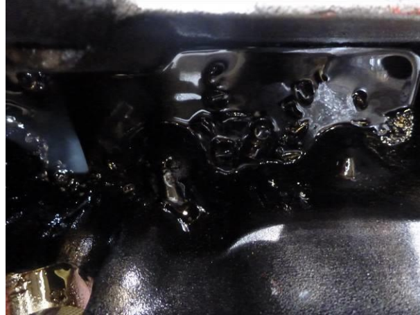
Figure 7. Broken gears in sump
