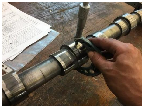
Figure 4. Inspected using a micrometer
