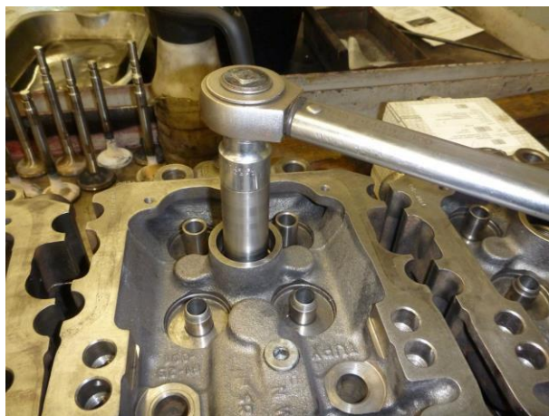
Figure 7. Sleeves, guides & plugs replaced
