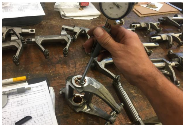
Figure 15. Crack detected and measured
